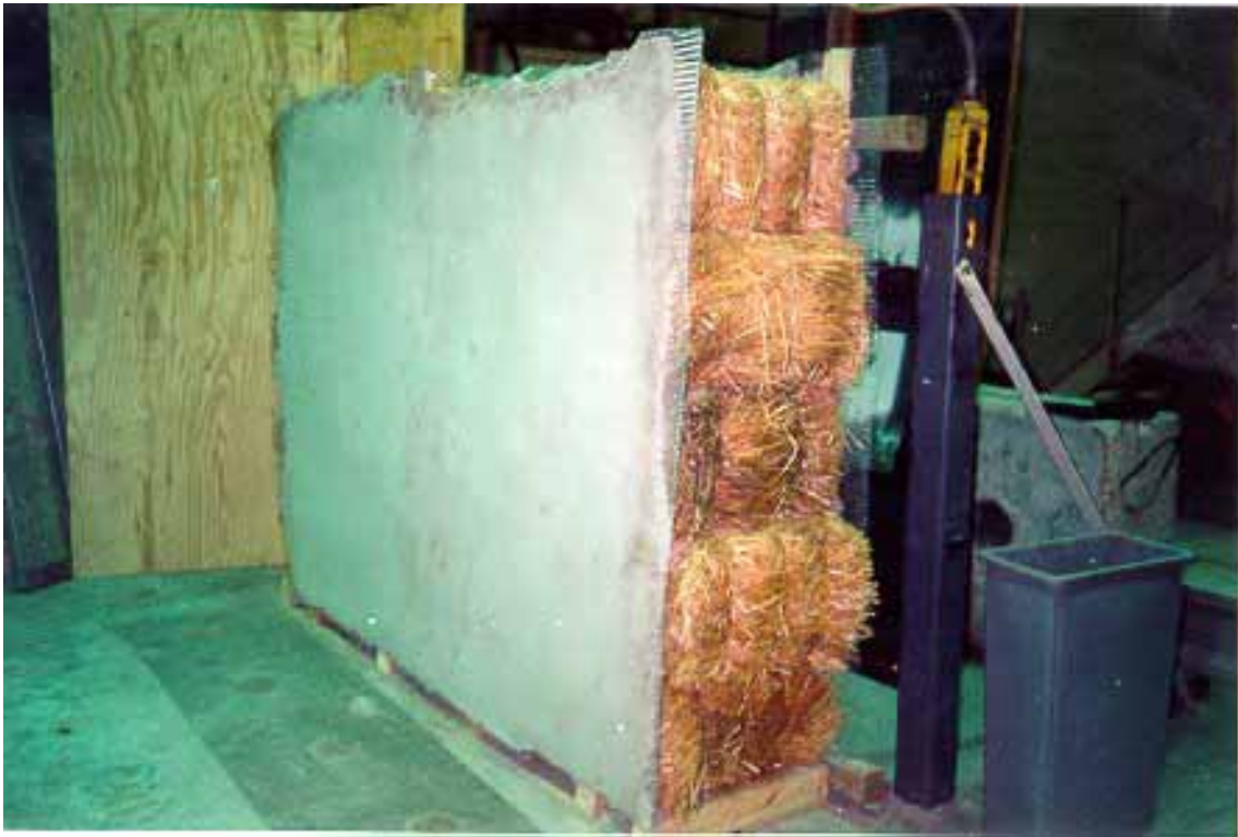
View of Impact Surface of Straw Bale Wall
