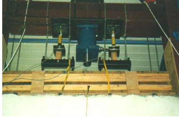
Figure 7: Hydraulic rams and top plate assembly for two-storey wall. (Photograph P. Florence)
