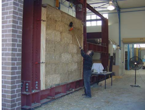
Figure 3: General view of earth rendered straw bale wall at time of trimming. (Photograph S.Overmeyer)
