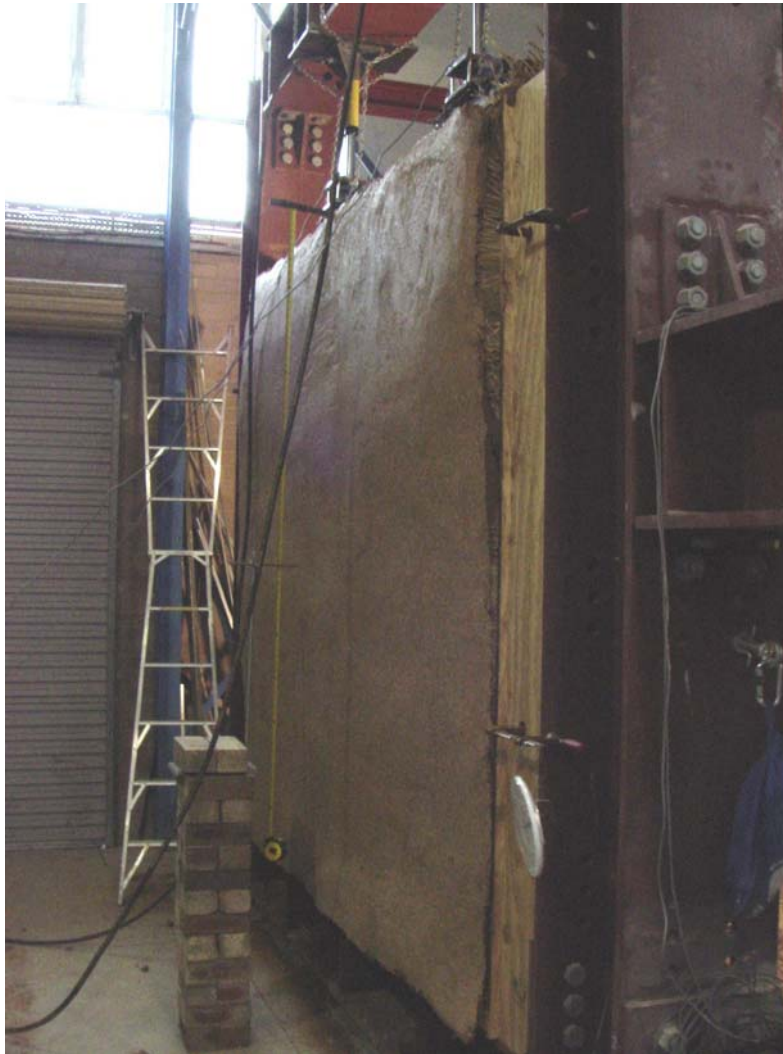
Figure 21: General view of the earth rendered wall in test frame. (Source S.Overmeyer)
