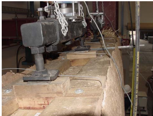
Figure 8: Hydraulic rams and top plate assembly for earth rendered wall (after test). (Photograph P. Florence)
