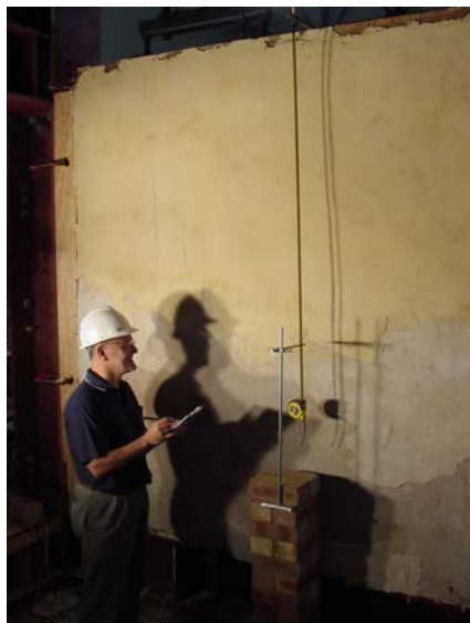
Figure 11: View of deflection measurement process for earth rendered wall. (Photograph P. Florence)
