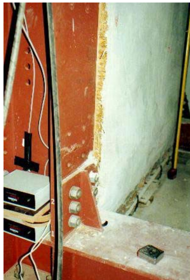
Figure 11: View of deflection measurement process for earth rendered wall. (Photograph P. Florence)
