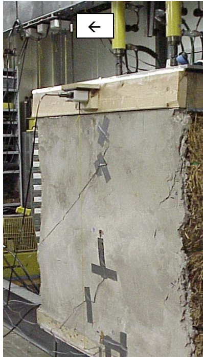
Figure 4.5 potentiometers attached to testing frame
